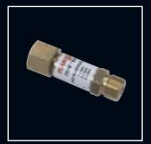
Where hose check valves are not is use, this device, having the same safety features as a Type 82 will add an increased level of protection to the ancillary equipment should a flashback occur. Available in 3/8" BSP, 9/16" UNF, 5/8" UNF and M16 inlet and outlet fittings.
