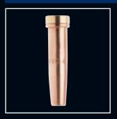
Designed for high speed oxy-propane machine cutting applications where productivity is a major issue. This two piece nozzle comprises a serrated inner and a copper outer. The special design allows for much faster cutting than PNM nozzles.
