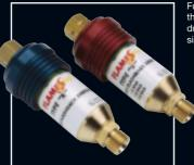
Fully re-settable, combines high flow rates with a pressure sensitive cut out mechanism, thermal valve, sintered stainless steel flame arresting element, gas non-return valve and a dust filter to ensure the utmost in safety, longevity and performance. Designed for use with single and multiple cylinders, manifolds and where larger flow rates are desirable.
