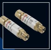
Comprising a sintered stainless steel flame arresting element, a thermal shut off valve, a gas non-return valve and a dust filter, this product is designed be used on single and multiple cylinder applications and tapping points and is intended to withstand a number of flashbacks and provide passive safety. Should the unit be subject to a severe flashback, the thermal element will be activated, completely isolating the regulator and gas source.
