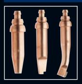
Available for cutting and gouging. Each nozzle is formed from copper rod and precision machined before swaging and finishing. The manufacturing process provides a quality product which allows accurate cutting due to the gas flow characteristics.
