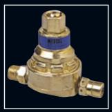
Available by special order only and one of the longest serving safety devices on the market, the Type 79 can be reset way of a pin mechanism, which promotes good practice when using equipment. Should the mechanism be activated, the whole gas system must be dismantled and the problem corrected before the device can be reset.
