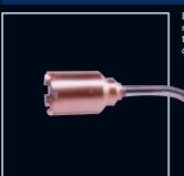
Designed to be used with oxy-propane and a Wescol Model 90 shank and superheating mixer and provide between 65,000 and easily in excess of 500,000 btu/hr dependant of the nozzle size and torch configuration. The castellated outer is made of high quality copper and the inner is brass.
