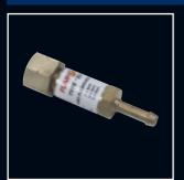
Designed to be fitted to the downstream end of hoses instead of hose check valve and connects to the inlet of hand equipment and to machine torches, this unit offers a non-return valve and flame arrestor which offers protection to the ancillary equipment in the case of a flashback arrestor. Available with 5mm, 6mm, 8mm and 10mm hose tail and 3/8" BSP, 9/16" UNF, 5/8" UNF and M16 inlet and outlet fittings.
