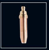
Wescol PNM nozzles consist of two precision machined parts, the splined brass inner and the copper outer. The design ensures gas flow characteristics that ensure the pre-heat flame sits at the nozzle face to give a precise cut.
