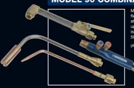
Manufactured in the UK to comply with BS EN ISO 5172. The Model 90 provides the flexibility that industry requires. The dedicated shank can be fitted with a cutting attachment and either ANM or PNM nozzles for heavy duty cutting applications (mild steel up to 200mm), or a mixer for gas welding and heating applications. A super heating mixer is available for use with super heating nozzles which will easily provide in excess of 500,000 btu/hr of energy where required.
