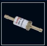
Where hoses are connected, this device, when placed inline and properly secured provides an additional level of safety for ancillary equipment. Comprising a non-return valve and flame arrestor, this device is available with 5mm, 6mm 8mm and 10mm tails.
