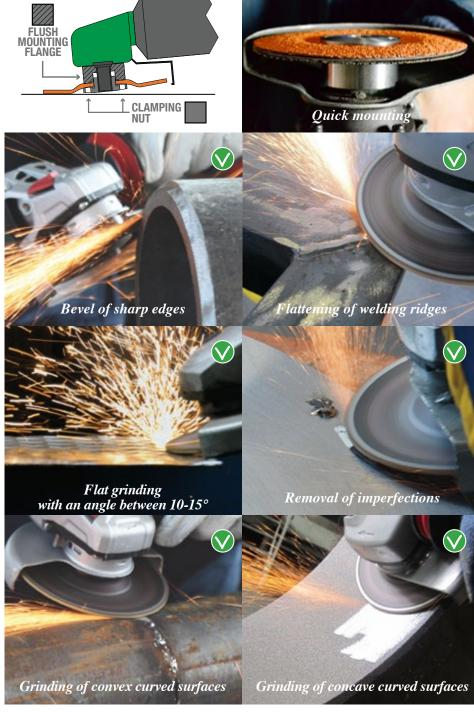
ASSEMBLY WITH FLUSH MOUNTING FLANGE KIT
