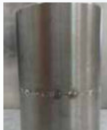
Pipe butt weld Ø 31.75 x 2 mm
