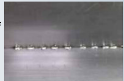
Corner spot welding thickness 0,6 mm
