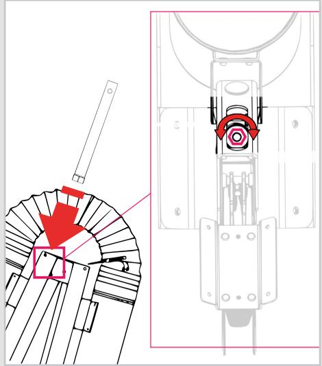
Turn the calibration tool **CLOCKWISE**.
