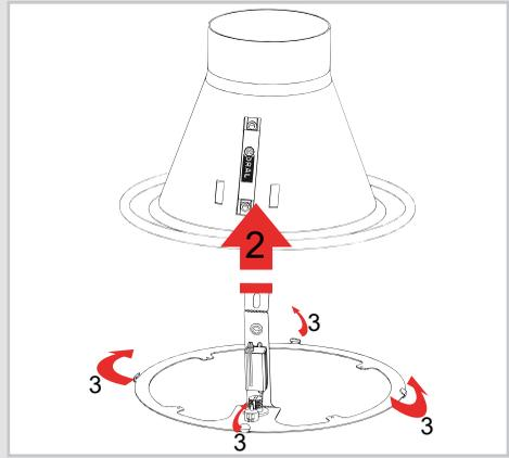
4) Fix the inner support of the frame with the handle fixing nut
