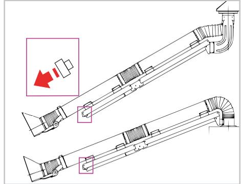
Insert the socket spanner in the recess housing the spring and fit it on the calibration nut. Insert a screwdriver from the side through the socket spanner and follow the instructions below.
