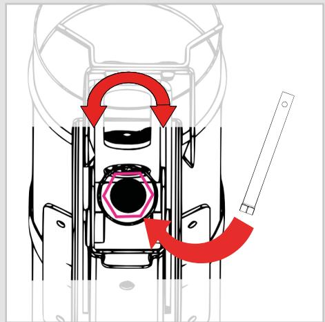
Turn the calibration tool **CLOCKWISE**.
