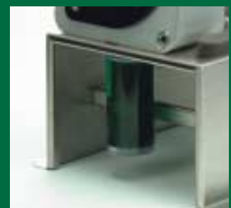
Sealed disposable container for toxic dust collection.
