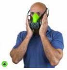
Inhale, pressing the palms of the hands against the filter; if the oronasal collapses towards the face it means that the half-mask is well positioned and tight. Otherwise, improve the positioning of the mask on the face and eventually increase the tension of the elastic bands.
