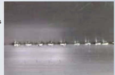
Corner spot welding thickness 0,6 mm
