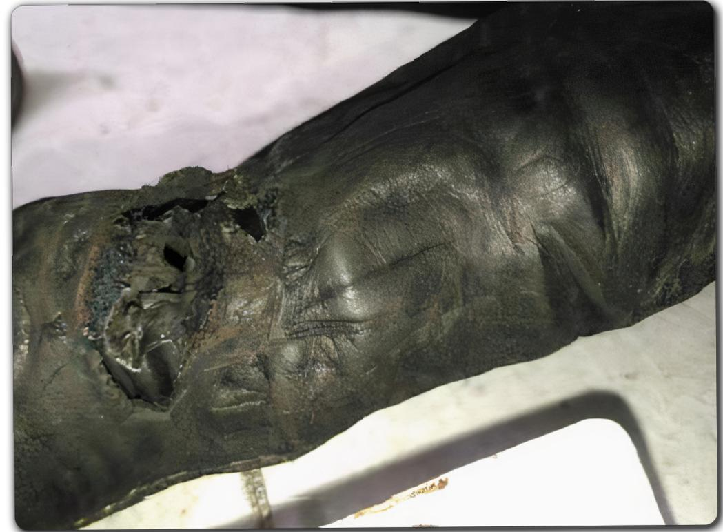
Excessive anti-spatter gel on welding application causes buildup of internal residues on the gun.
