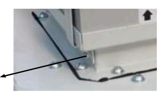
UNSCREW THE FOUR FASTENER AND REMOVE THE BRACKET.
