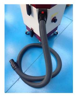
Connect the opposite side of the hose to the extraction Y connection of the welding torch
