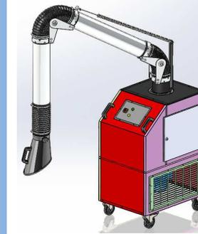
For the replacement of carbon filters, unscrew the side vents on the sides, on which are threaded, as shown above. You have to pull out the old filter from the grill then insert the new one.
