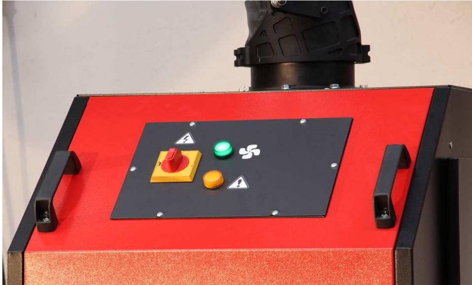
The machine is equipped with an electrical panel which acts as control panel and as container for the protection devices of the electric motor.
