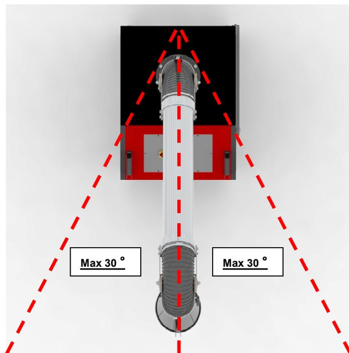
The use of the suction arm outside the recommended range may cause the machine to tip over. In fact, when movements are carried out along the longest side of the machine the force exercised is such as to move the barycentre and act as a lever lifting and/or tipping over the air cleaner in the direction of the operator moving the arm.
