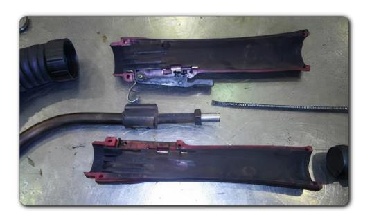
Gun with wet residue inside it, increasing the weight for the welder.
