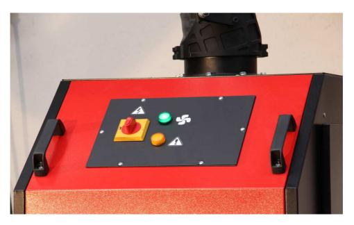
The machine is equipped with an electrical panel which acts as control panel and as container for the protection devices of the electric motor.
