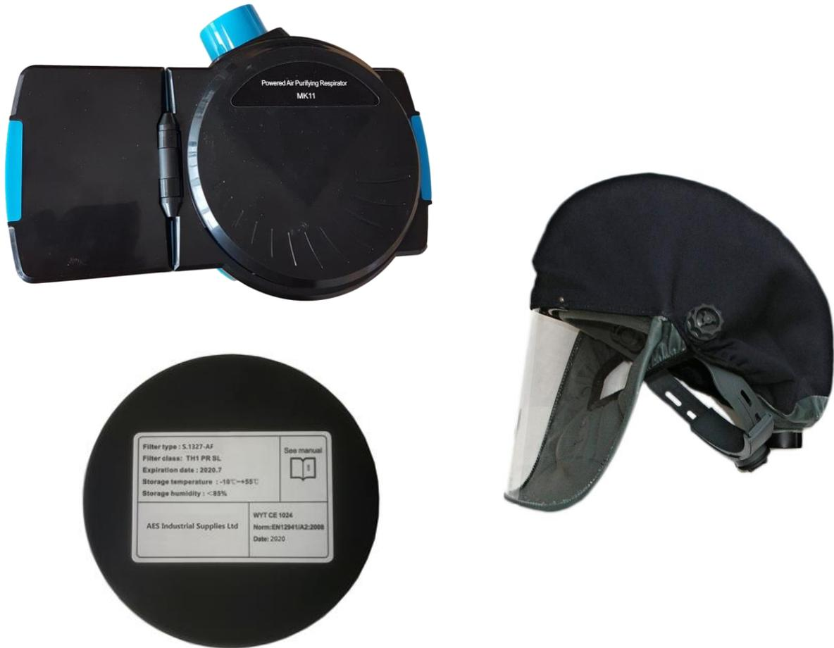
The powered filtering device incorporating a hood Max-Arc MK11 equipped with a particle filter S 1327-AF TH1P R SL protects the respiratory system of a user against harmful aerosols in the air according to the instructions of the manufacturer.
