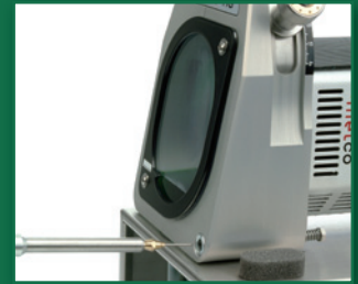
Precise adjustment of the stick-out
