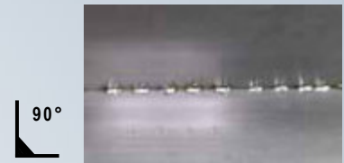
Corner spot welding thickness 0,6 mm
