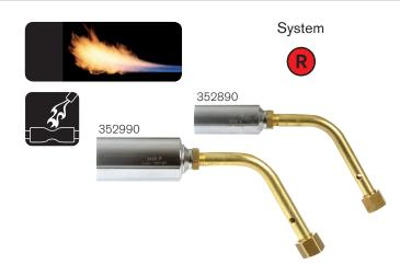
• Soft flame design ideal for cable work and other heat shrinking applications • Soft flame burners with sweeping, powerful yellow and blue soot-free windproof flames • Fresh air sucks in and keeps the burner head cold to minimize the risk of burning the shrink material • To heat the sleeves efficiently but still soft enough not to overheat the shrink material • For direct connection to Sievert Pro handles • Working pressure 2 bar
